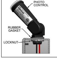
POSSIBILITY of water entering the unit around the wires. This includes not installing the unit on the bottom of the junction box. 4) Wire the photo control per the Wiring Diagram below.
